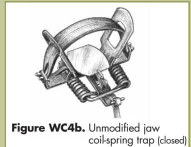
**Figure WC4b.** Unmodified jaw coil-spring trap (closed)
